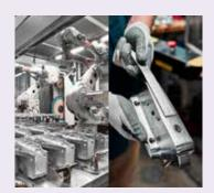
Kason 58 latch bodies ready for robotic polishing (left) and after final assembly (right).
