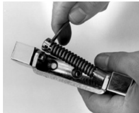
2. Slip bushing over hexagon pin on mounted hinge; then insert adjustment pin into adjustment bushing assembly.
