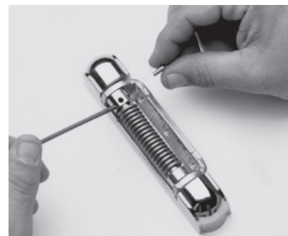
3. Adjust tension; then insert stop pin in hole of adjustment bushing assembly.
