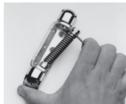
2. Place throughst washer and bushing over hexagon pin on mounted hinge. Insert adjustment pin into adjustment bushing assembly. Grasping adjustment pin, compress spring and place adjustment bushing assembly over round pin.
