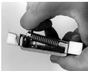
3. Grasping adjustment pin, compress spring and place adjustment bushing assembly over round pin.
