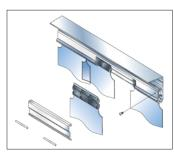
Maximum-duty system made of heavy gauge aluminum extrusions. Specify "JM" for center cut out.
