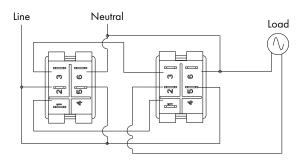
Three-way switch application "NIGHTLIGHT" or indicator always "ON"
