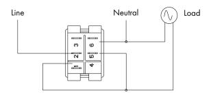
Single switch application indicator is "ON" when light is "ON"
