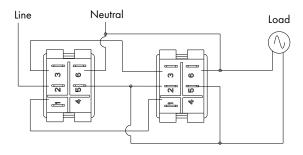
Three-way switch application indicator is "ON" when light is "ON"
