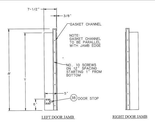
Fig. 10 Completed Jamb Assembly
