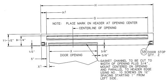
Fig. 9 shows a completed Header Assembly of a Manual Single Doorware System
