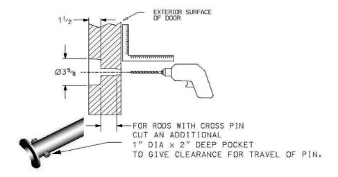
3. Hollow out the insulation within the cut-out area to the 1-1/2" depth. Hole will accept recessed housing as shown below. Check fit by placing recessed housing in large hole on interior side of door aligning center hole with 3/4" through hole. Push rod must move freely through insulation.
