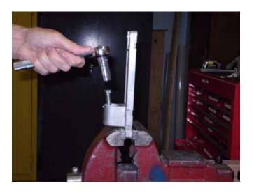
Drive the bolt into the cam.
