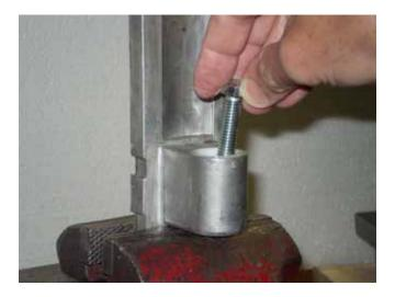
Obtain 3/8 bolt to be used as puller for removing cam. Insert the bolt into the hole in bottom of cam.
