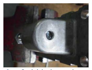
Do not allow the bolt end to go past the cam material into the metal body of the hinge flange.
