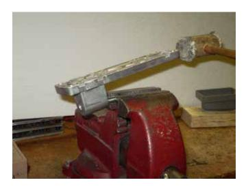
Secure the bolt head in a vise, tap the flange body gently with a hammer.
