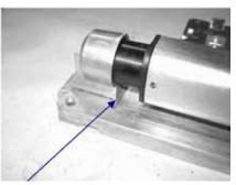
Note final position of top cap, base is nearly flush with cut-out in flange
