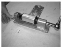
While tightening nut on screw put downward force on end cap base as shown
