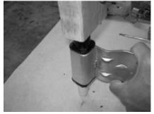
Orient top bearing so that drill hole aligns with hole in strap & tap to seat
