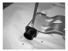
Use drill motor to fasten bearings in place with self drilling screws
