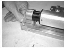
As nut is tightened top cap should move smoothly in slot
