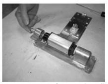
Insert top cap into flange and install center screw, if necessary tap screw to align
