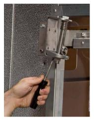
Hinge cam block adjusts with philips head screwdriver.
